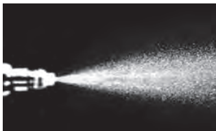
Injector spray pattern after P.i. treatment.
