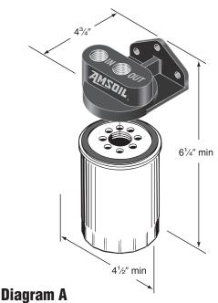
MINIMUM AREA NEEDED FOR REMOTE MOUNT FITTINGS, AND SMALLEST SPIN-ON OIL FILTER ELEMENT.
