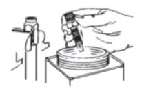
2. Oil inside of hose and nipple threads liberally with oil. Do not oil hose cover.
