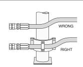
3. Protect from hazardous environment Keep hose away from hot parts. High ambient temperature will shorten hose life. If you can not route it away from the heat source, insulate it.
