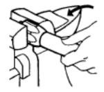
1. Place socket in vice and screw in hose counter-clockwise until hose bottoms. Back hose out 1/2 turn.
