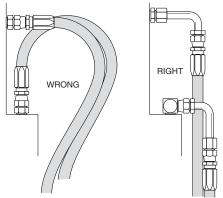
Use elbows and adapters in the installation to relieve strain on the assembly, and to provide easier and neater installations that are accessible for inspection and maintenance.
