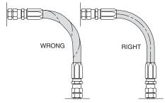
Do not twist hose during installation. This can be determined by the printed layline on the hose. Pressure applied to a twisted hose can cause hose failure or loosening of connections.
