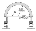
Maximum bend radius is measured on the inside bend of the hose. To determine minimum bend, divide the total distance between ends (B length) by 2. For example 8 = 6, minimum bend radius = 3.
