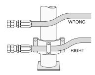
Keep hose away from hot parts. High ambient temperatures will shorten hose life. If you can not route it away from the heat source, insulate it.
