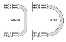
Keep the bend radius of the hose as large as possible to avoid collapsing of the hose and restriction of flow. Follow catalog specs on minimum bend radii.
