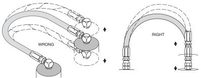
Make sure relative motion of the machine components produces bending rather than twisting of the hose. Hose should be routed so that the flex is in the same plane as the equipment movement.
