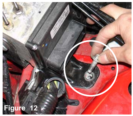
Figure 13 Remove the m8 bolt on top of the strut tower mount.
