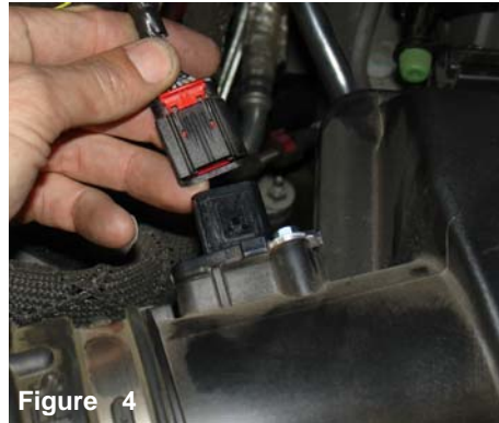
Figure 4 Mass air flow sensor harness clip is disconnected.
