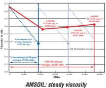
Class 8 Kenworth T600 tractors with Series 60 Detroit Diesel engines. Conventional oil changes: 20,000 miles Oil changes extended to 56,343 mile (average) with AMSOIL.
