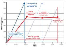
AMSOIL: minimal cylinder, crankshaft wear Class 8 Kenworth T600 tractors with Series 60 Detroit Diesel engines.
