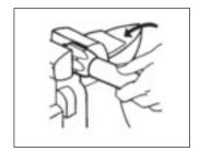
Place socket in vice and screw in hose counter-clockwise until hose bottoms. Back hose out ½ turn.
