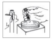
Oil inside of hose and nipple threads liberally with oil. Do not oil hose cover
