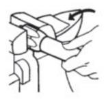
Place socket in vice and screw in hose counter-clockwise until hose bottoms. Back hose out ½ turn.
