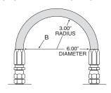
Maximum bend radius is measured on the inside bend of the hose. To determine minimum bend, divide the total distance between ends (B length) by 2. For example B = 6, minimum bend radius = 3.
